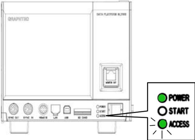
(12) The firmware update is completed when the blinking of access LED was stopped.
